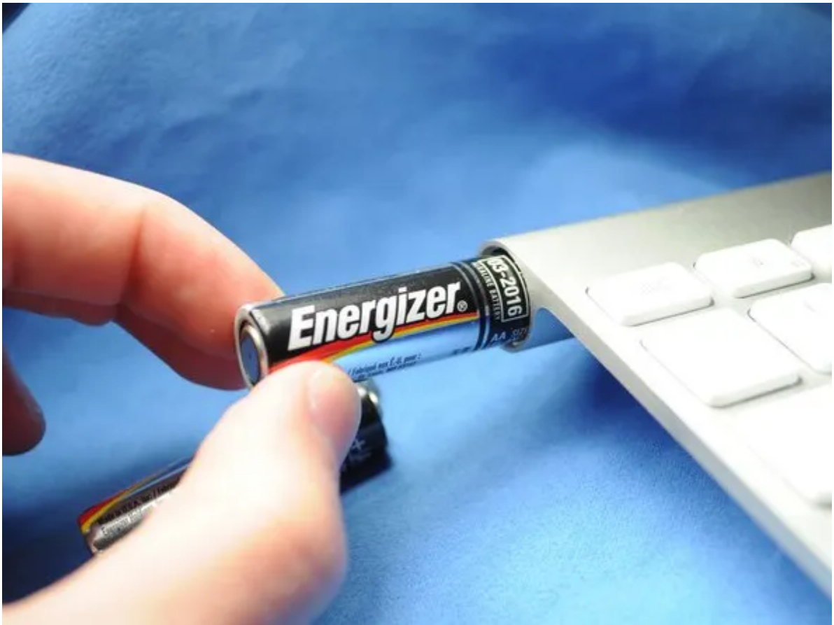
Caption: A new battery being inserted in the battery cover in a wireless keyboard.
